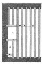
Floor with simple joists
