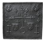
Picture #4 : Gothic fireback : Decorations (border and inside lines) were made with cabletwist placed inside the mould.
